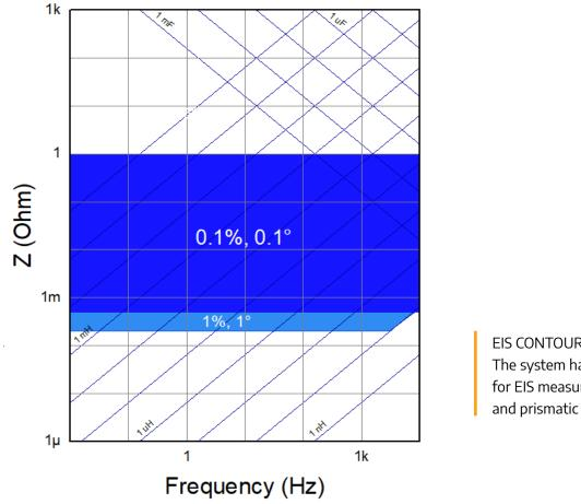
EIS CONTOUR MAP The system has been optimized for EIS measurements of pouch and prismatic cells.
